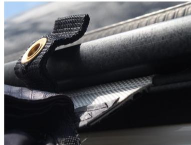
8. Take the awning piping and slide it through the awning channel, until the awning is in the desired position on the vehicle. We recommend using a 'Drive Away Kit', as it will make this process much easier.
